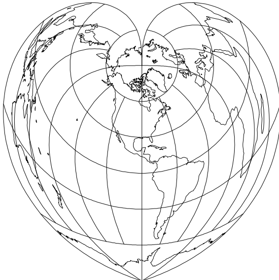
Figure 46: Werner projection, with shorelines and 30^\circ graticule. Central Meridian 90^\circ W ( +proj=bonne +lon_0=90w +lat_1=90n ).
