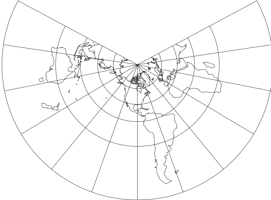
Figure 37: Lambert Conformal Conic projection, with shorelines and 30^\circ graticule. Central Meridian 90^\circ W. and standard parallels at 20^\circ N and 60^\circ N ( +proj=lcc +lon_0=90w +lat_1=20n +lat_2=60n ).
