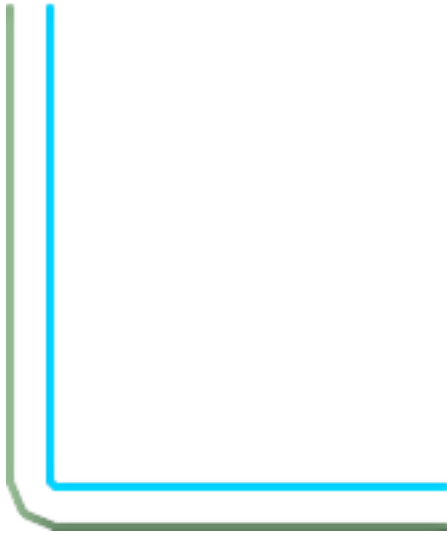
15, 'quad_segs=4 join=bevel' shown with original line
