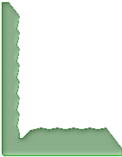
Concave Hull of L points at target 80% convex hull area
