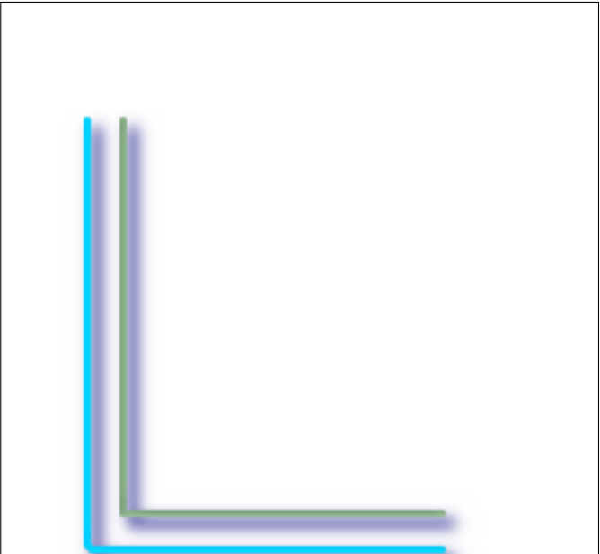
-15, 'quad_segs=4 join=round' original line and its offset -15 units
