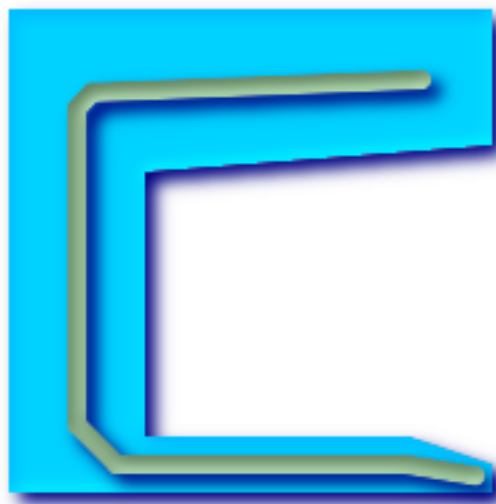
A polygon and its approximate medial axis
