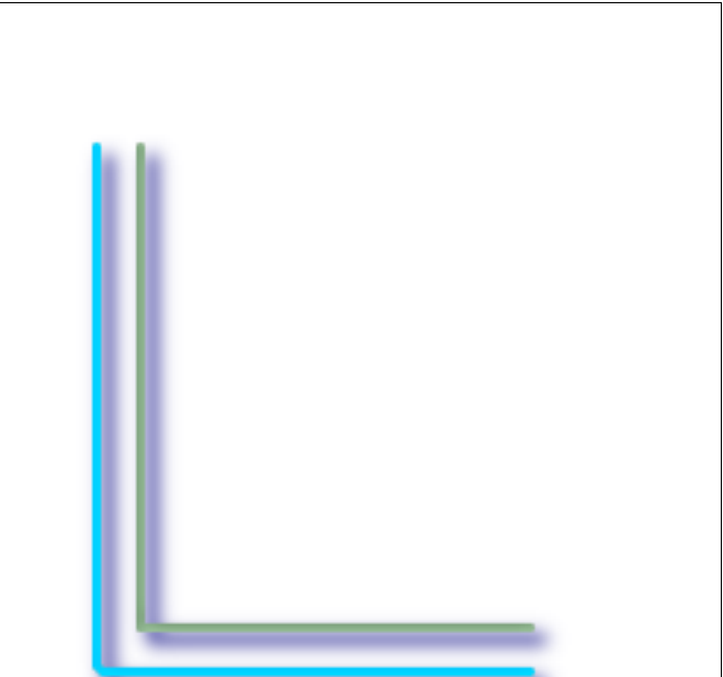
-15, 'quad_segs=4 join=round' original line and its offset -15 units
