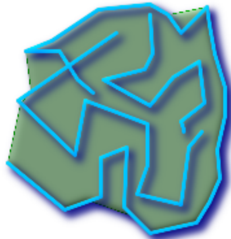
multilinestring with overlaid with Concave hull of linestrings at 99% target -- first hop
